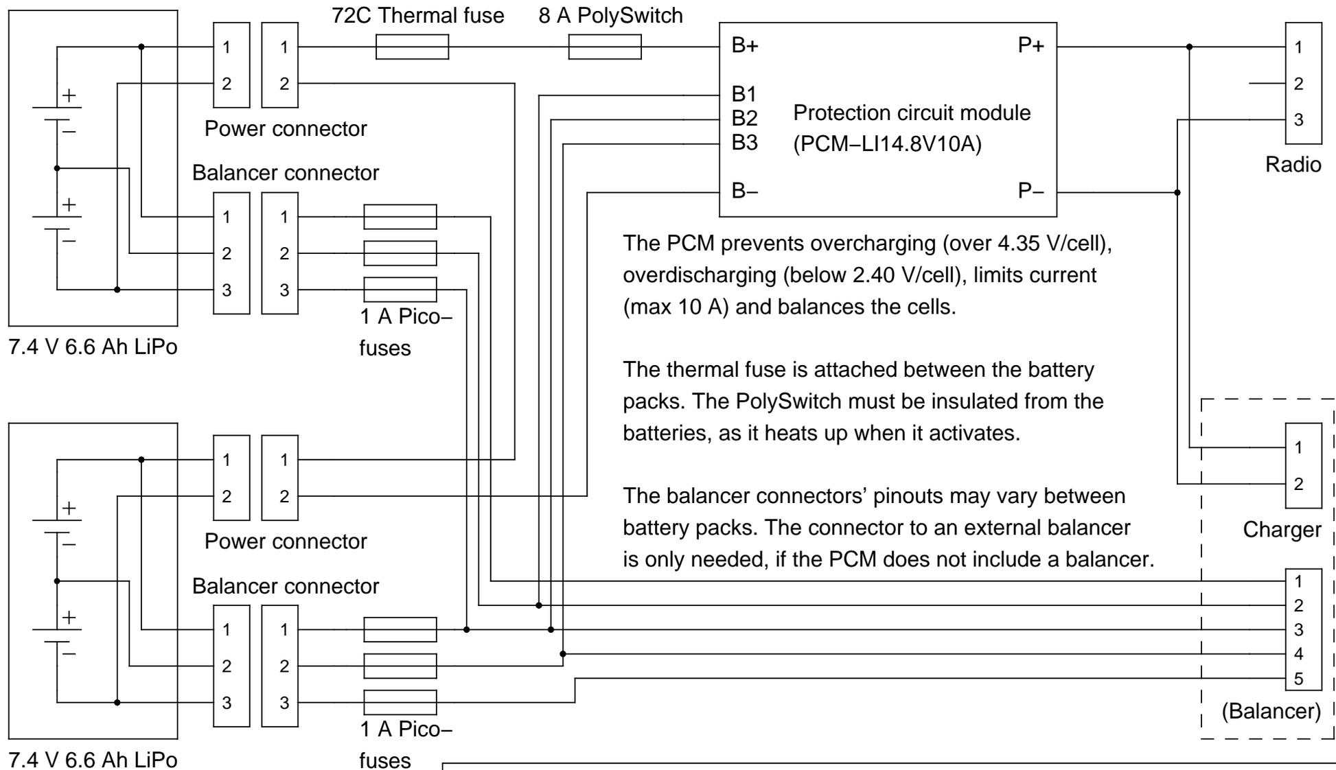
LiPo-batteries and protection circuits for the FT-897
