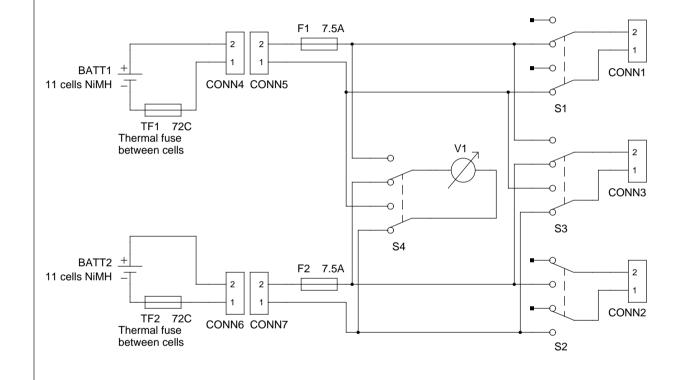
S1 and S2 are two–pole ON/OFF switches that switch CONN1 and CONN2 to BATT1 and BATT2, respectively. S1 is shown in "ON" position, S2 is shown "OFF". S3 is a two–pole ON/OFF/ON switch that switches CONN3 to BATT1, BATT2 or OFF. S3 is shown in "BATT2" position. S4 is a returning two–pole (ON)/OFF/(ON) switch that switches volt meter V1 to BATT1, BATT2 or OFF. S4 is shown in "BATT2" position. All switches are two–pole in order to provide complete isolation when switched "OFF".
